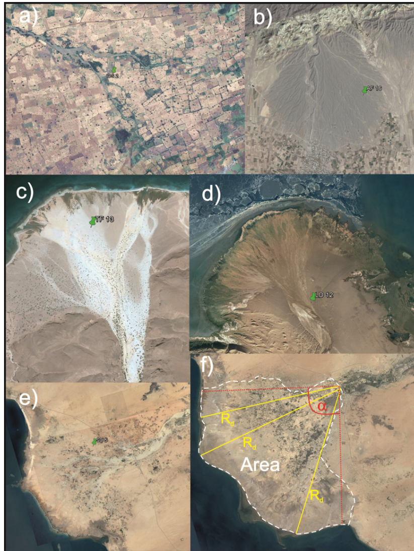
Figure 1 The main typology of distributive systems considered in this study: a) distributary system, sensu stricto ; b) alluvial fan; c) fan delta; d) lacustrine delta; e) sea delta; f) the main geomorphic parameters measured: area is the area of the distributive system body; R_d is the radius; \alpha is the apex angle.
