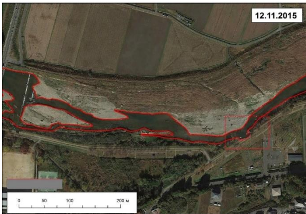
Figure 5 Section 18 (sub-zone 3) of the lower reach of the Niida River before (A) and after (B) extreme flood. Legend: 1 – eroded part of the bank of the Niida River protected by concrete embankments; river channel position before extreme flood, 01.06.2015; 3 – river channel position after extreme flood, 12.11.2015. As can be seen the road on the right bank is completely washed out
