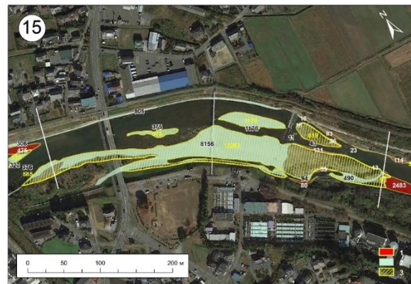
Figure 7 The bank erosion (1), in channel deposition (2) and floodplain sedimentation (3) zones formed after extreme flood at the section 3 (plain sub-reach) within the wandering (braided) type of the Niida River channel.
