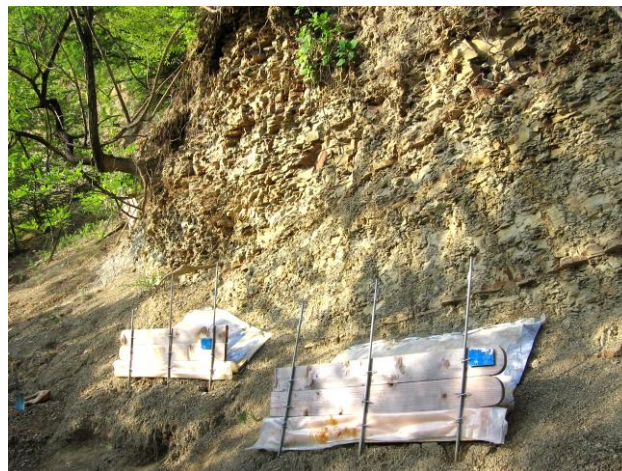
Fig. 5. Semi-open erosion plots for flysch rockwall retreat measurements (photo: Matija Zorn)
